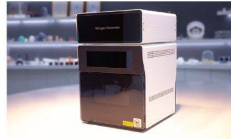
Fig. 7. Tera Harz Cure Machine with a nitrogen generator.
