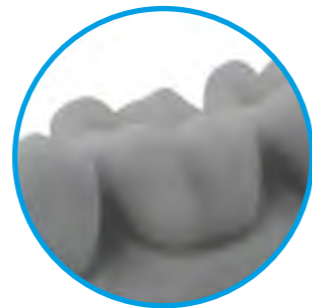
Surface at 50 microns Z-resolution
