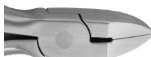
Hard Wire Cutter, 15° 15° offset tip enhances access in difficult areas. Designed to cut hard wires. 0,56 mm x 0,71 mm 678-103
