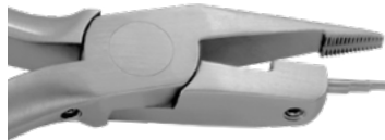
Omega Loop Forming Pliers Graduated cone is designed to form precise omega loops: .045", .060" and .075" <= .022" x .025" (.56 mm x .64mm) 678-303 Replacement Blade for 678-303 QTY: 1 678-002 1/8" Set Screw and Hex Key for 678-303 QTY: 1 678-018
