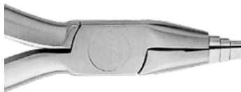
Old Style Loop Pliers Provides optimum accuracy and precision in forming and closing loops with one cylindrical three-step beak and one triangular beak. <= .022" x .028" (.56mm x .71mm) 678-324
