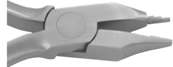
Tweed Loop Forming Pliers Loop forming pliers with .055", .075" and .090" diameters for creating bull and helical loops in wires. <= .022" x .028" (.56mm x .71mm) 678-306
