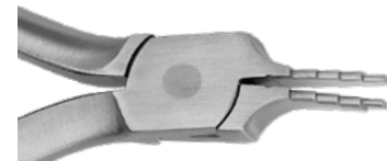
Nance Loop Forming Pliers For precise forming of loops in four lengths: 3, 4, 5 and 6 mm. Groove at base aids in closing loops. <= .022" (.53mm) 678-319
